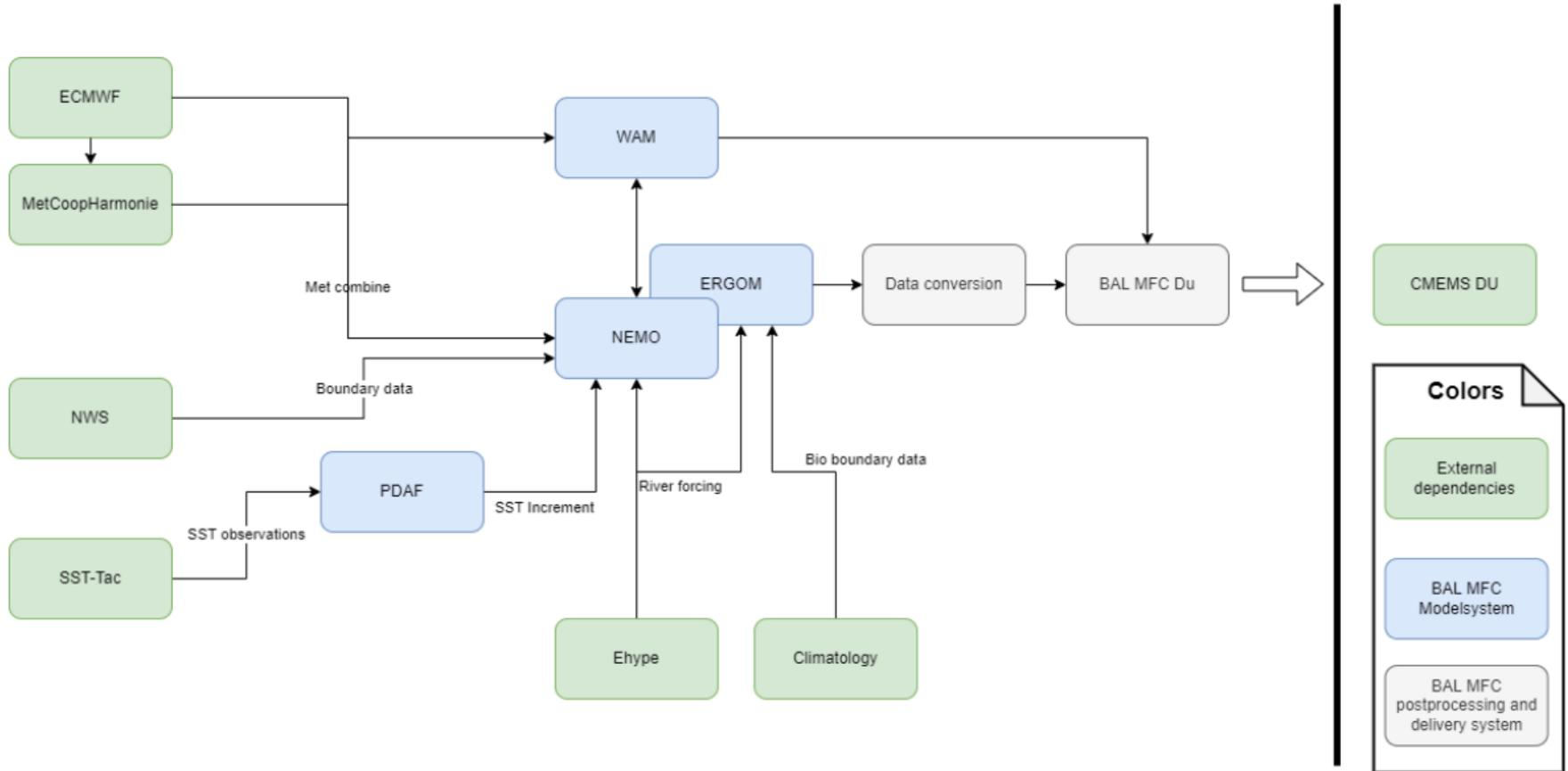
**Figure 3.1** process chart of the BAL MFC model system
